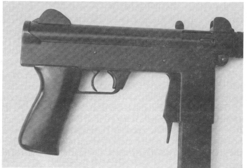
Above: Removable trigger assembly of the MP83A1.
