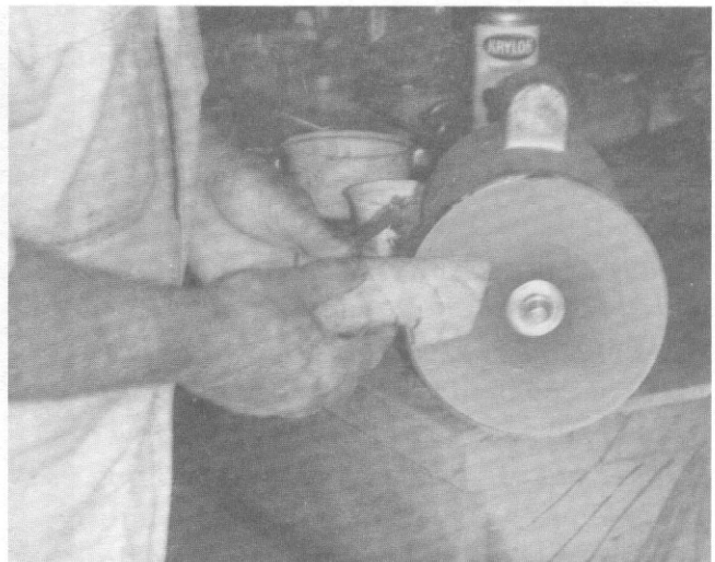
Grip can be shaped almost to final contour using disc sander.
