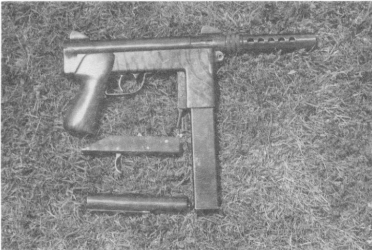
Left: Completed MP83A1 shown with interchangeable bolt and trigger assembly, which allows conversion to open-bolt operation.
