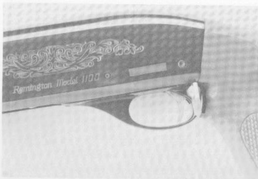
Another left side view showing selector lever on "semiauto" position.
