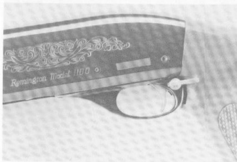
View showing the selector lever mechanism set on "safe" position with the shotgun fully assembled.
