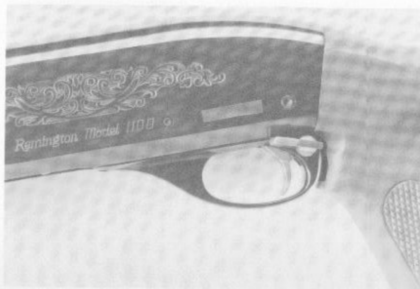
View showing selector at "full auto" position.
