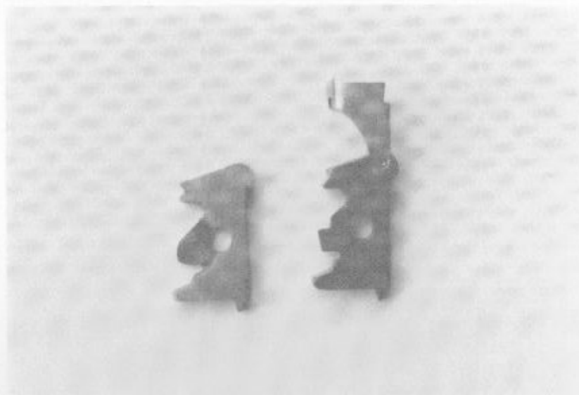
Comparison between the original sear (left) and the modified sear with the extension riveted in place (right).
