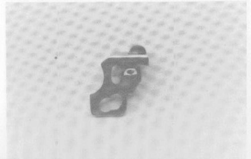
Detailed right side view of the automatic tripper without its spring and guide rod.
