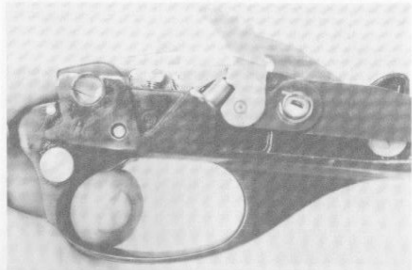
View showing the relationship of parts after the first shot is fired, the hammer recocked, and the link shoulder not pressing the tripper on rearward recoil. Note how the trip nose slightly parallels and rides well above the sear extension step ready for reengagement.
